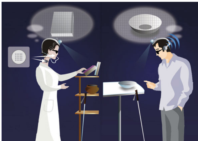
Fig. 18.2 The general concept of sensory substitution (SSD) and a typical visual-to-auditory and visual-to-tactile setup. SSDs typically include a visual capturing device (for example camera glasses), a computational device transforming the visual input into either a tactile or an auditory display using a simple known transformation algorithm, and an output device, transmitting this information to the user. The right side illustrates an example of an auditory SSD (such as The vOICE; Meijer, 1992) transmitting the sensory-transformed information using headphones, and on the left side is an example of a tactile device which may transmit the tactile information via an electrode array targeting the tongue (such as the TDU, Bach-y-Rita et al., 1998) or another skin surface, in this case presented on the neck (copyright of image, by Amir Amedi)
